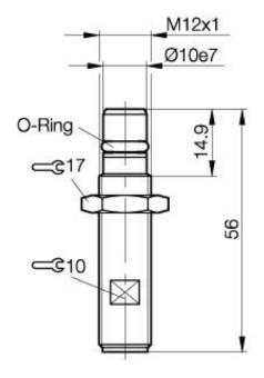
**Inductive Sensors** BES 516-300-S 265-S 4-D M12x1 x 56 normally-open Sn=1,5mm shielded pressure rated to 500 bar
